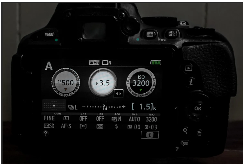
When the f-number is smaller (e.g., 1.8, 3.5, or 5.6), the aperture is wider. (Image by Mat Coker)
