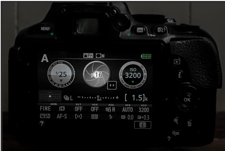
When the f-number is larger (e.g., 11, 16 or 22) the aperture is narrower. (Image by Mat Coker)
